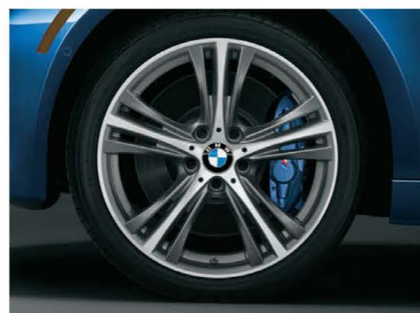
Star Spoke light alloy wheels (Style 407) 19 x 8.0 front, 19 x 8.5 rear; and 225/40 front, 255/35 rear run-flat 1 performance tires 2,3
