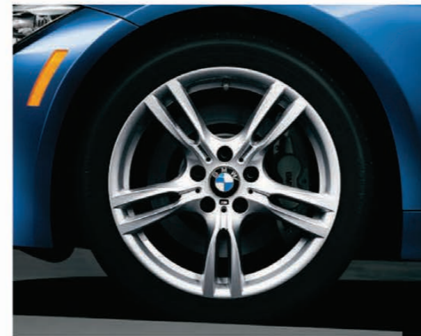
Star Spoke light alloy wheels (Style 400M) 18 x 8.0 front, 18 x 8.5 rear; and 225/45 front, 255/40 rear performance run-flat 1 tires 1,2,3 18 x 8.0; and 225/45 run flat 1 all-season tires 2
