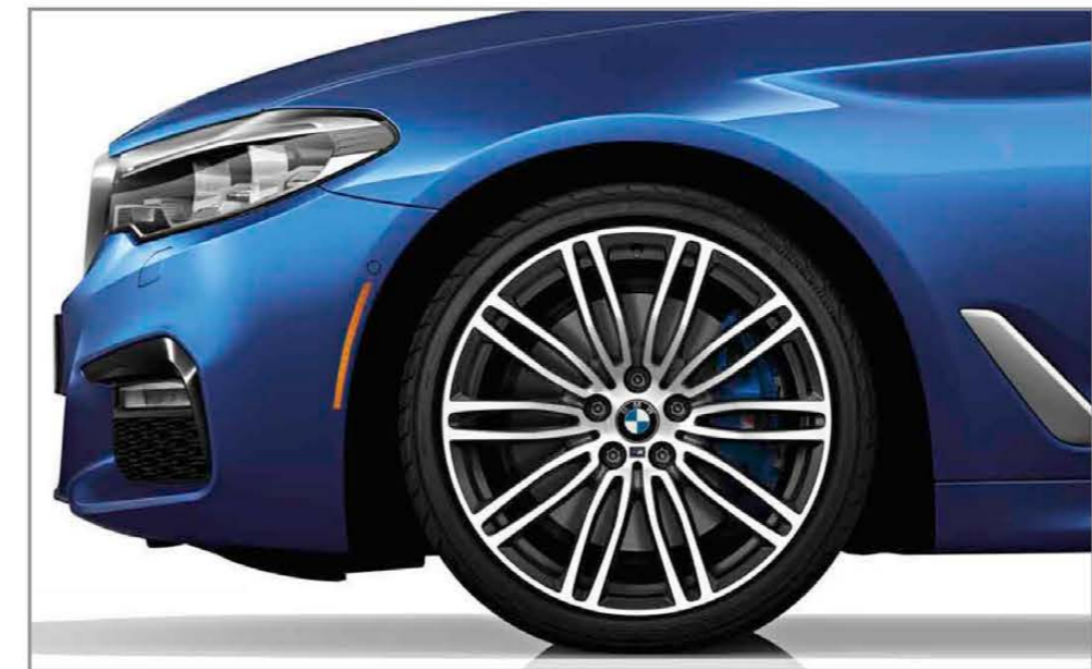
Double Spoke light alloy wheels (Style 664M), 19 x 8.0 front, 19 x 9.0 rear; and 245/40 front, 275/35 rear run-flat performance tires 1,2
