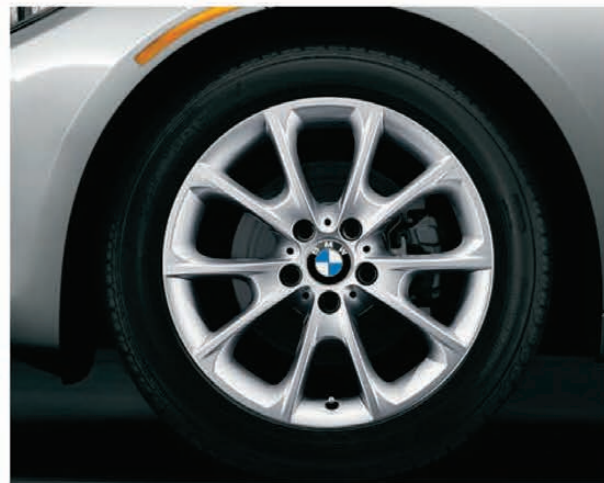
V Spoke Orbit Gray light alloy wheels (Style 398) 18 x 8.0 front, 18 x 8.5 rear; and 225/45 front, 255/40 rear performance tires 1,2,3
