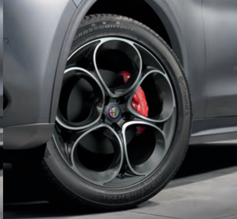
20-inch Sport 5-hole aluminum wheels Available on Ti, Ti Sport and Ti Lusso
