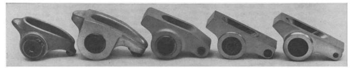
custom replacement rocker arms are generally stronger than those offered by the factories. In addition to possessing superior strength, most custom rockers are lighter in weight and feature needle-bearing-equipped trunnions. Some have roller tips to reduce friction and wear, and a few are even adjustable to make valve adjusting simpler than ever. There are quite a few rockers on the market, so let's take a look at some of them.
