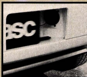
Above left: Rear wheel skirts are slotted halfway down to vent underbody pressure. Skirts remove easily for tire changing. Above right: Electrically operated license plate hides gas cap.
