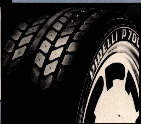
The P700's outer tread blocks are oriented to resist the forces induced by simultaneous braking and cornering.
