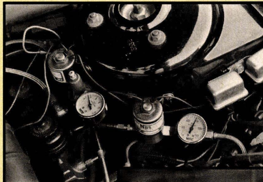
Simple nitrous-oxide system produces copious power but demands care. Excessive heat stops N 2 O flow, and low-rpm use produces backfires and shattered air cleaners.
