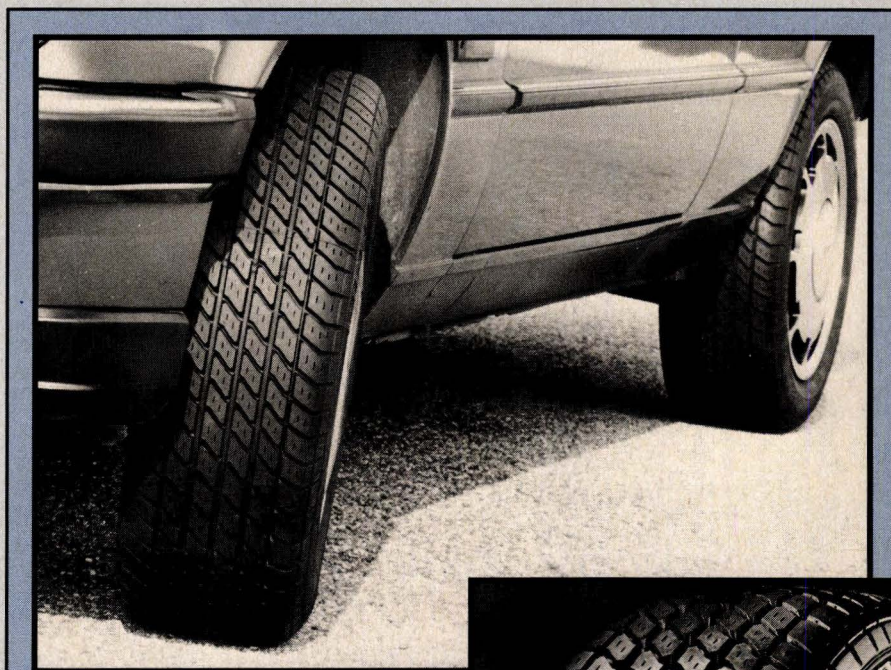
The P600's new tread provides improved aquaplaning performance at high autobahn speeds.
