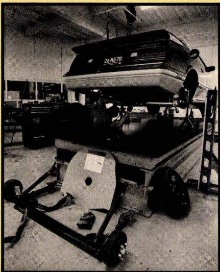
A surface plate facilitates precise assembly.
