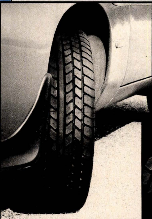
The P700's outer tread blocks are oriented to resist the forces induced by simultaneous braking and cornering.
