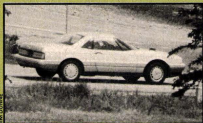
Cadillac's 1987 front-drive, two-seat Allanté, a convertible with a removable hard top, will be powered by Caddy's own 4.1-liter, injected aluminum V-8, mounted transversely. Designer Pininfarina will build the bodies in Italy and ship them to GM's Poletown plant near Detroit for final assembly. Price: near $50,000.
