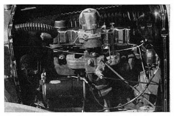
The 3%-inch bored, 153-cubic-inch Chevy II mill with Powerglide is a comfortable fit in the '27 Ford's engine room. Red wire wheels shod with 5.00 x 16 Goodyears up front and dropped axle give Bo's sedan proper rake combined with 7.50 x 16 rear weenies. Interior is strictly "yesterday" except for S-W gauges in engine-turned dash, boasts vintage steering wheel. The rear view sums it up in a word character!
