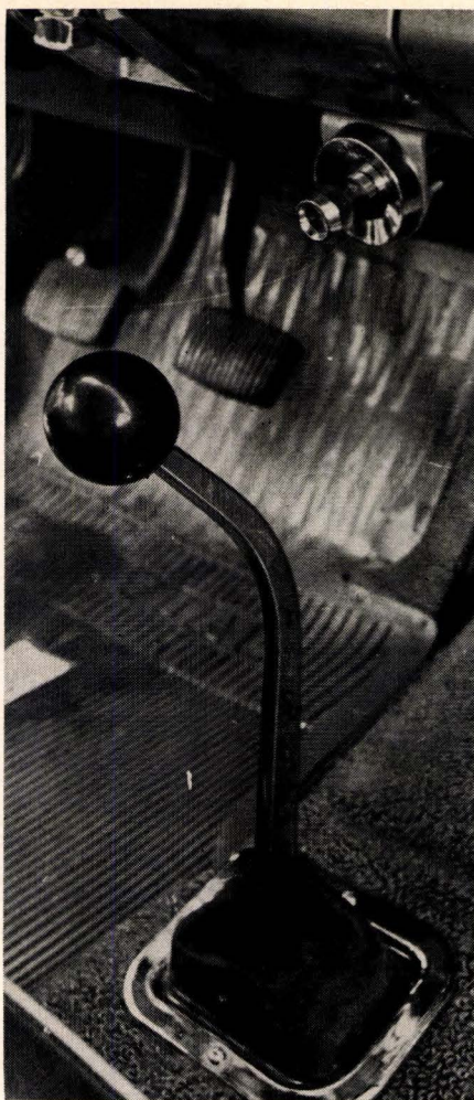
The unbeatable Hurst-Campbell floor shift and heavy-duty linkage setup is standard equipment with the four-speed box and 421 engine combination.
