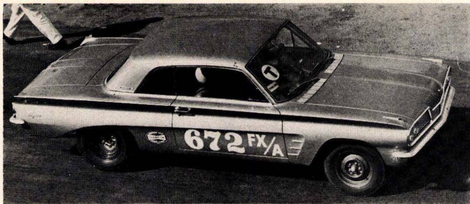
Proffitt's class-winning FX/A Tempest was crammed with 487 inches of screaming Pontiac. Charged through the lights at 117.27 mph, with 12.37 e.t. Car had big Pontiac driveshaft and rear axle. Engine was built by Thompson Enterprises.
