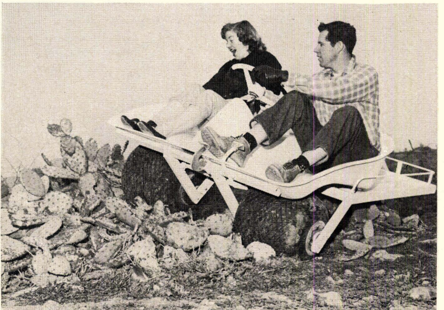
Even prickly pear cactus is no obstacle to the flabby Terra tires. The pressure is so low that no suspension is necessary.
