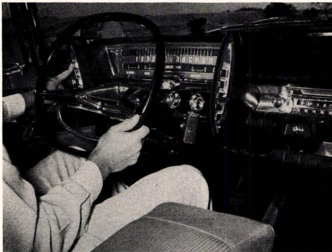
The mammoth control console relies on the Chrysler pushbutton theme. Note the squared steering wheel.
